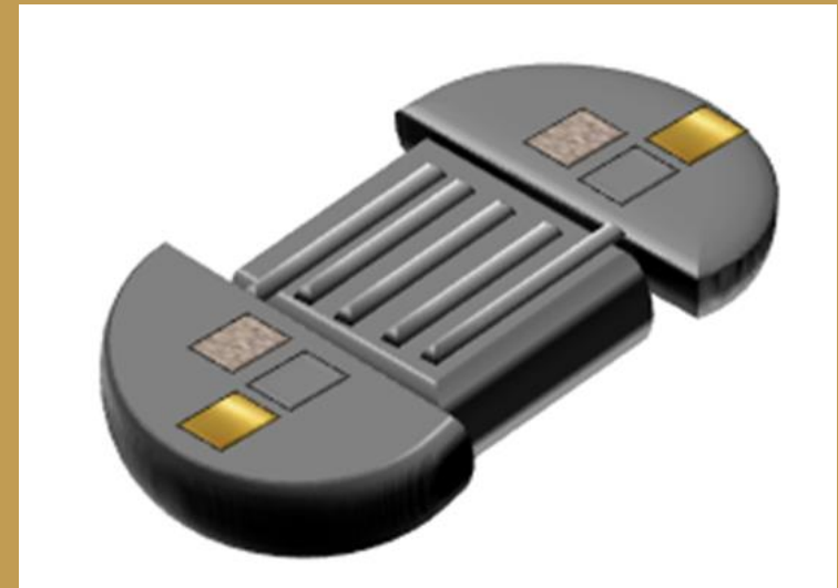
Figure 1: 3D rendering of micromachined oscillator
