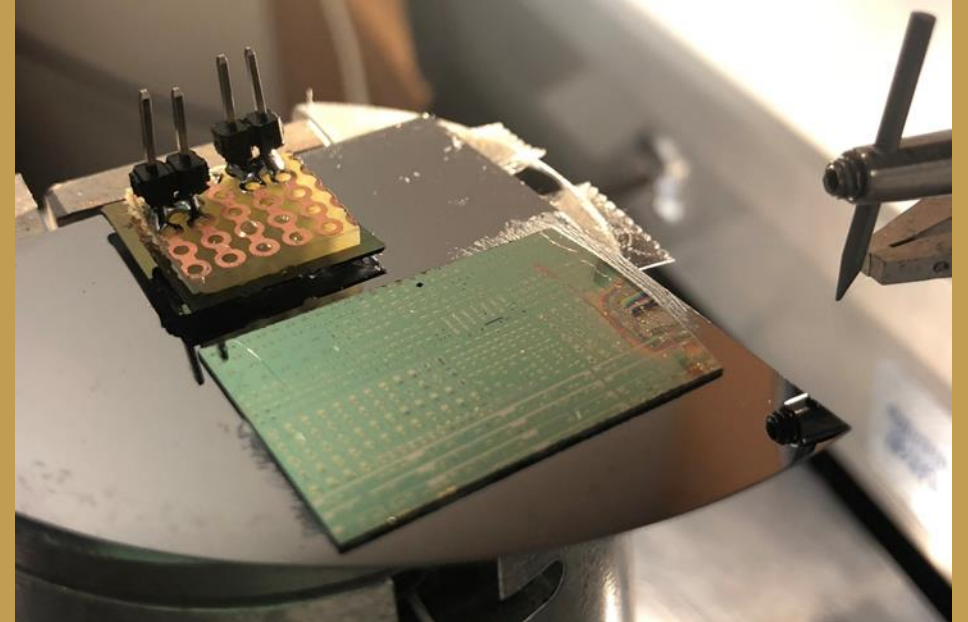
Figure 2: Fabricated oscillators on silicon
